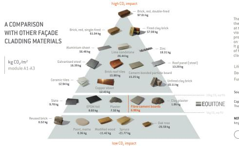
The Construction Material Pyramid was developed by the Centre for Industrialised Architecture [CINARK] at the Royal Danish Academy in 2019. It is a way of visualising the carbon emissions associated with the production of different materials. The pyramid focuses on the product stage [life cycle phases A1 - A3]. It gives an impression of the global warming potential of fibre-cement boards in general compared to other cladding materials.
