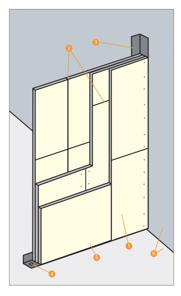
Solid Partitions El 30 to El 240 Integrity and Insulation in both directions
