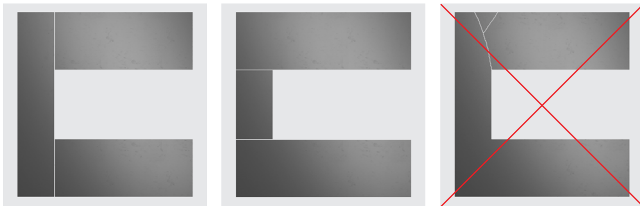
Correct mounting of Hardie® Panel & Hardie® Architectural Panel at windows, doors and openings.
