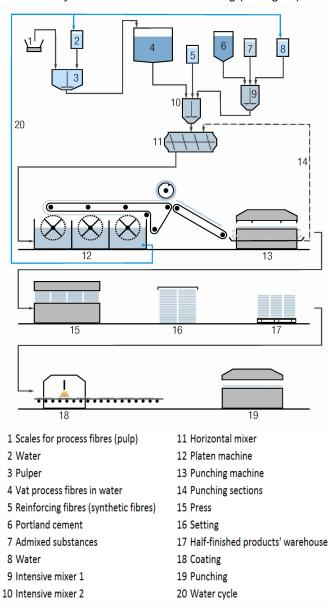
The raw materials are treated with water to a homogeneous
