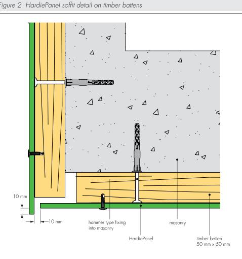
Figure 2 HardiePanel soffit detail on timber battens
